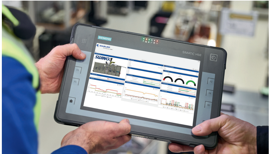
Fig. 3. Portable comfort panel: the Gabler dashboard developed in cooperation with Siemens visualizes machine and process data via the open, cloud-based software system MindSphere
