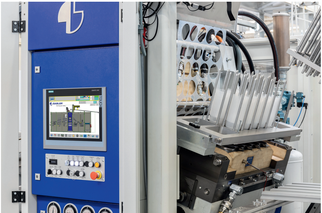
The extended machine functionality of the new thermoforming line can be safely controlled by a single operator using the Simatic HMI comfort panel © Siemens
